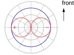
**Figure 2:** Polar response of a the stereo microphone composed of coincident omnidirectional and bidirectional (or *figure-of-eight*) microphones.
