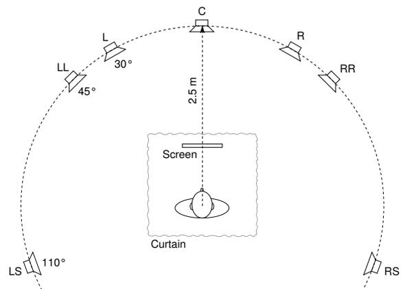
**Figure 1:** Playback setup consisting of seven loudspeakers: left (L), right (R), center (C), left-of-left (LL), right-of-right (RR), left surround (LS) and right surround (RS). This setup was symmetrically placed with respect to the width of the room and was hidden from the subject by an acoustically transparent curtain. A computer flat screen was used as a response interface.
